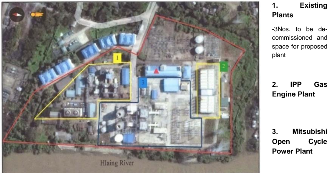
Figure 1-1: Existing Plant Layout
