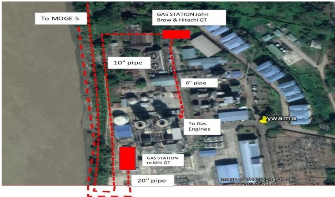
Figure 3-5: Gas Pipelines in the Plant Area
